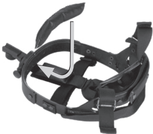
Figure 4-1. Removal and Installation of Browpad
