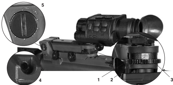
Figure 3-5. Windage and Elevation Adjustment
