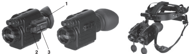
Figure 2-5. Dual Bridge Adapter
