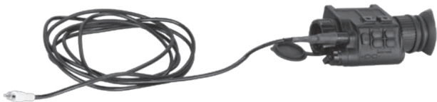
Figure 2-2. Attaching Video Cable
