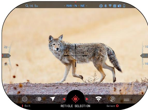
To enter the RETICLE SELECTION menu, open the Shortcut Carousel by pressing the OK button and select the RETICLE SELECTION menu with the LEFT and RIGHT buttons.
