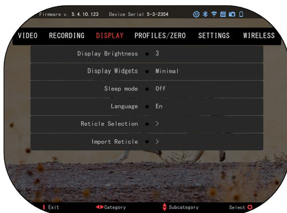
DISPLAY BRIGHTNESS. Gives you a 1 to 5 numerical selection, with 1 being the dimmest and 5 the brightest. It is recommended that you use the brightest setting during the day for optimal performance.
