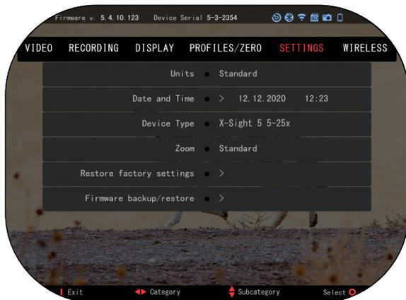
To enter the System Settings, open the Shortcut Carousel by pressing the OK button. Select the wrench icon with RIGHT or LEFT buttons.
