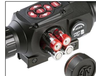
Do not over tighten as it will be difficult to remove the next time you replace batteries. But make sure that the Red O-Ring is not visible, after the battery cap is reinstalled. This will prevent shut off issues due to recoil.
