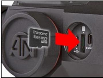
3. To lock when inserting card in the slot, push it with a thin object (a small coin, paper clip, toothpick, etc.).
