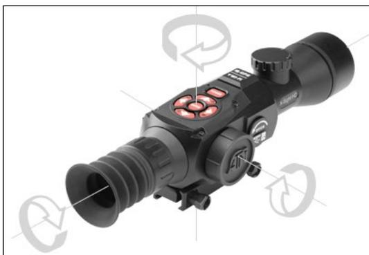
When the compass needs to be calibrated the word "CAL" appears instead of the Compass Scale. To calibrate you should rotate the device in three axis as pictured on the left.
