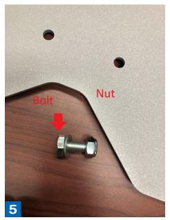
Repeat the process with the interior nuts and bolts. Align the floor stand over the interior bolts. Secure the base plate to the floor stand.
