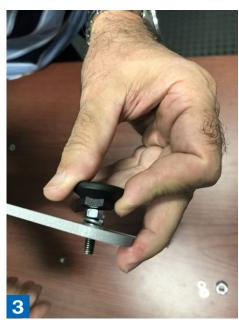
Install the stabilizing pegs on the four corners of the base plate making sure it is leveled.
