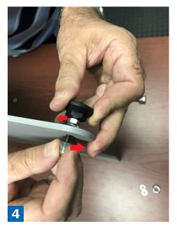
Secure the "acorn" nut turning clockwise while holding the stabilizing peg and rotating it counter clockwise.
