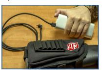
Place the battery with the USB cable attached in to the rifle pouch battery compartment.
